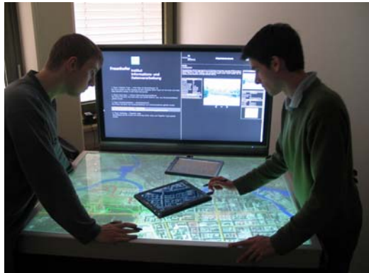
Fig. 5. Digital situation table consists of a horizontal work table, Fovea-Tablets ® offering local high resolution, and a vertical screen displaying additional information
