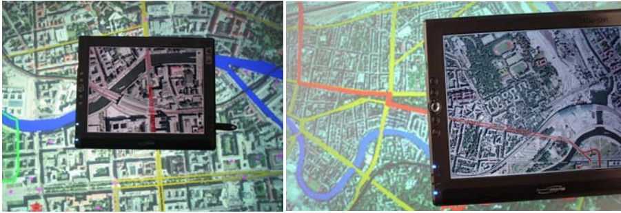
Fig. 6. A Fovea-Tablett ® positioned on the work table offers a local view with high resolution
