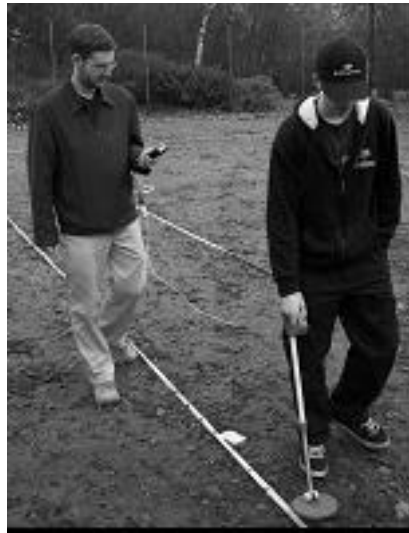
Fig. 5. Searching for Targets using metal detector and GPS linked via WLAN to command post
