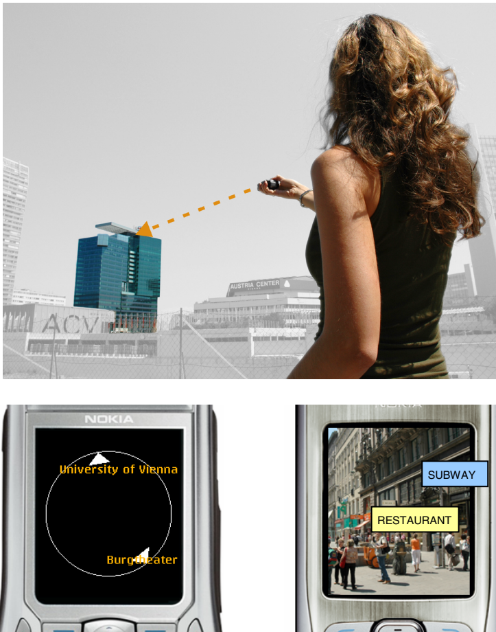
Fig. 1. Forms of mobile spatial interaction. Top: a ‘geo-wand’, bottom left: a ‘smart compass’, bottom right: ‘augmented reality view’.
